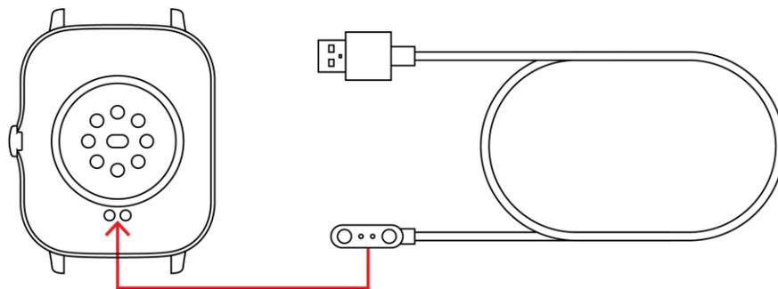
**NOTE:** Do not have the charger connected to AC and the magnets touching any metallic surface, this will create a high heating of the cable and will damage it.
