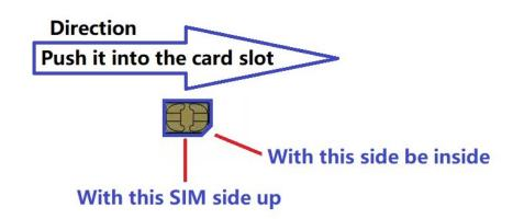
You can hear a tiny sound once the Nano SIM card has been inserted into the SIM card slot and into the right position.
